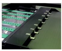
Servo driven feed- and discharge grippers running over precise linear bearing rails. The feed gripper takes the sheet from the camera registration position and places the sheet in the center under the screen. The position of the print table is automatically adjusted to the sheet size.
