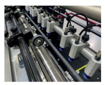
The proven single-sheet front-pick-up feeder can handle the most difficult substrates and securely places the sheets on the infeed table. The belt system transports the sheet to the gripper pick-up position. Optional "just-in-time" sheet cleaning can be installed.
