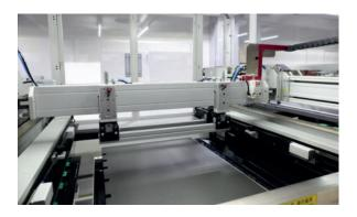
The squeegee assembly runs in 90° angle to the sheet transport. Squeegee and flood coater are quick and easy to insert. Squeegee and flood coater are driven by servo motor and securely run in linear bearing rails.
