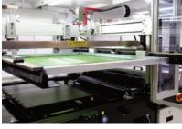
The retractable screen frame outside of the machine body makes cleaning and/or corrections comfortable. After push back there is no need for new registration, production can continue without any further interruption.
