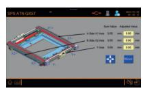
If necessary, minor further screen registration corrections can be given a numeric input on the large size color display (HMI).
